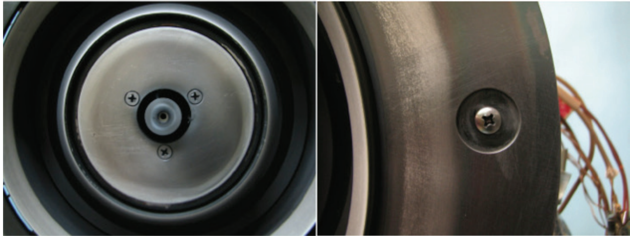
Figure 17 Left: Photograph of the inner front pole and cathode keeper after the wear test. Carbon deposition was evident over most of the inner front pole. A ring of discoloration was evident on the cathode keeper, similar to erosion patterns observed with the NSTAR ion thruster discharge cathode assembly. However, machining marks were still visible after the wear test, so it is not clear if significant erosion was occurring here. Right: Photograph of the outer front pole after the wear test. Various bands of backspattered carbon were evident on the outer front pole. The light colored region was easily removed with a razor blade after the wear test.
