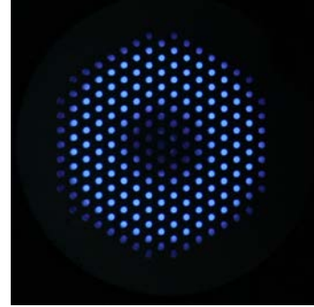
Figure 6. Photograph image at the x-y plane of \mu 1 in plasma-discharging operation.
