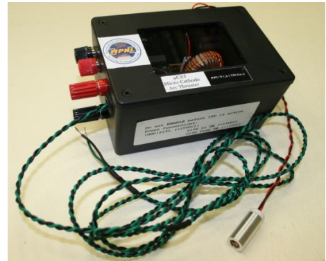
Figure 12: 1-Channel \mu CAT Subsystem (2013, THG2.2/PPUV7x)
