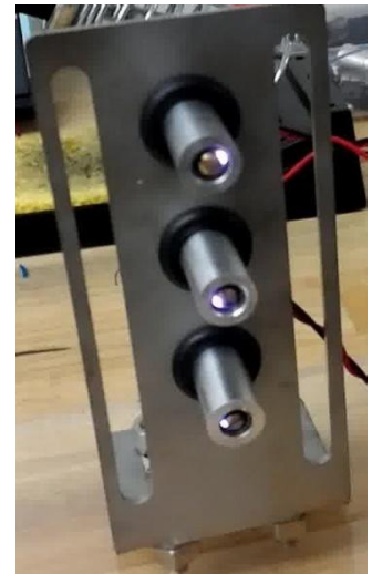
Figure 13: First Light Test. Three \mu CAT thrusters firing at the same time
