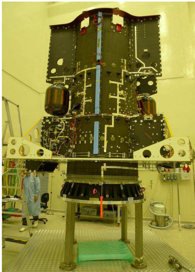
Figure 6 Xenon tanks integrated on the propulsion module
