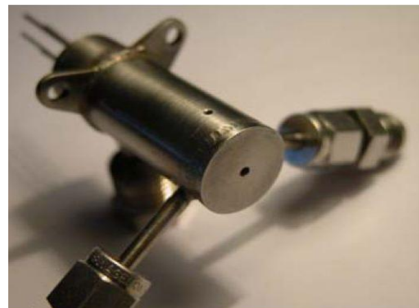
Figure 2. Alta's XR-50 first generation resistojet, optimized for low weight (60 g).
