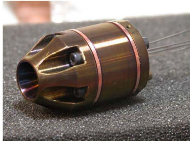
Figure 1. Alta's first xenon resistojet prototype designed for 50 mN of thrust at 50 W.
