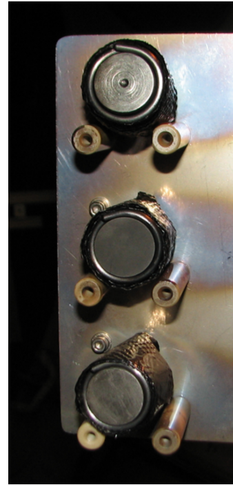
Figure 3. Stainless steel (top), graphite (center) and boron nitride (bottom) heated samples used for calibration.
