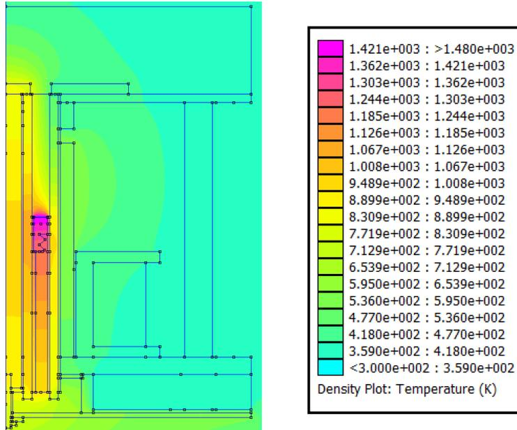
Figure 4. Axisymmetric thermal simulation of the WET-HET operating at 1 kW. The axis of symmetry is on the left hand side
