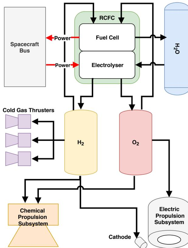
Figure 1. A fully integrated spacecraft water system architecture. Water is electrolysed so that it can be used for the electrical propulsion system, chemical propulsion system, and fuel cell.
