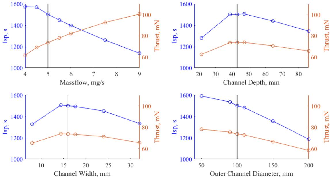
Figure 2. PlasmaSim sensitivity analysis for an SPT100 HET at constant power. The black line represents the actual value.
