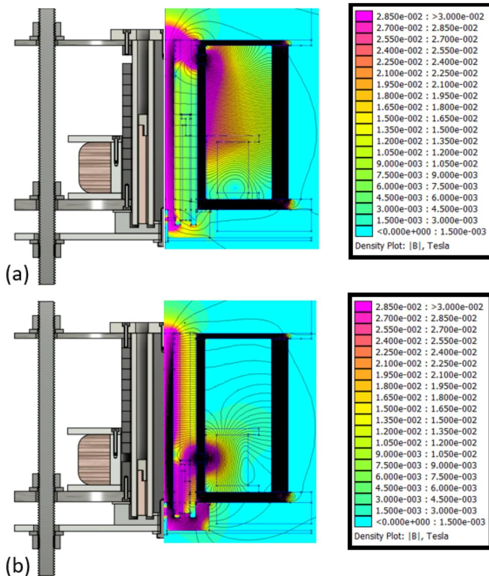
Figure 5. The WET-HET showing different magnetic field configurations, with superposition of magnetic modelling. The configurations in 5a shows minimum magnetisation region with all rings in the downward position. The configuration in 5b shows all rings in the raised position, producing the longest possible magnetisation region. Note that in 5b a smaller anode has been installed, increasing the channel depth to the maximum.
