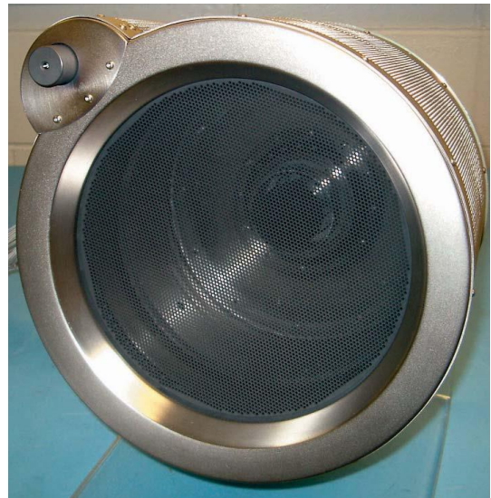
Figure 18. T6 electron-bombardment ion thruster.
