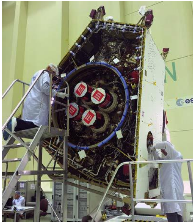
Figure 11. Electric propulsion thruster and pointing mechanism configuration.
