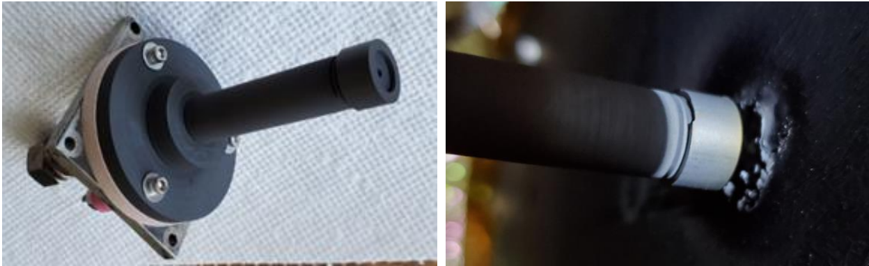
Fig. 22. Photograph of the Tubular 4 cathode assembly before testing (left) and after testing (right). Note the deposits that formed on the anode just downstream of the keeper tip. The keeper tip was fabricated with a cap that could be removed to allow different keeper orifice plates to be used. The keeper ID was reduced and the cathode tip to keeper orifice plate distance was increased in an attempt to reduce arcing at startup on Ar.
