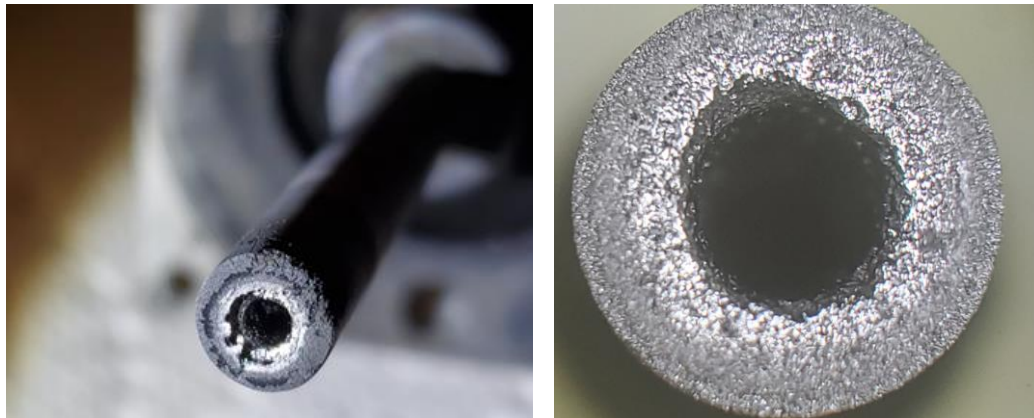
Fig. 19. Photograph of the graphite cathode tip (left) of the Tubular 3 cathode after testing on Ar and iodine for 2.3 hr and 25 hr, respectively. Damage to tip was very likely caused by arcing during starting on Ar. Photograph of the downstream end of the cermet insert (right) after removal from the cathode.
