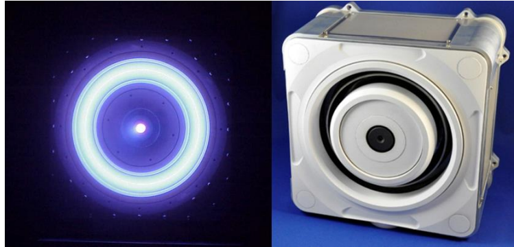
Figure 14: BHT-8000 operating on Krypton propellant (left), with center-cathode plume visible; static (right).
