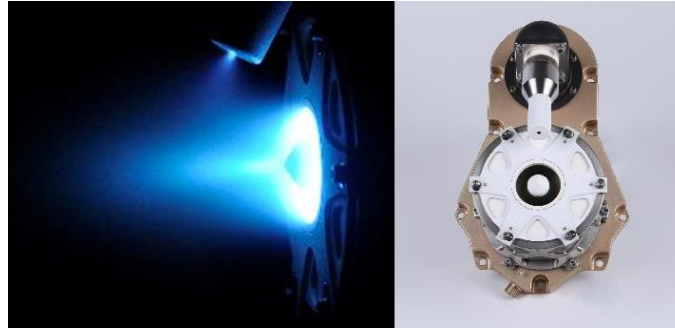
Figure 10: BHT-200 operating on Xenon propellant (left); static (right)
