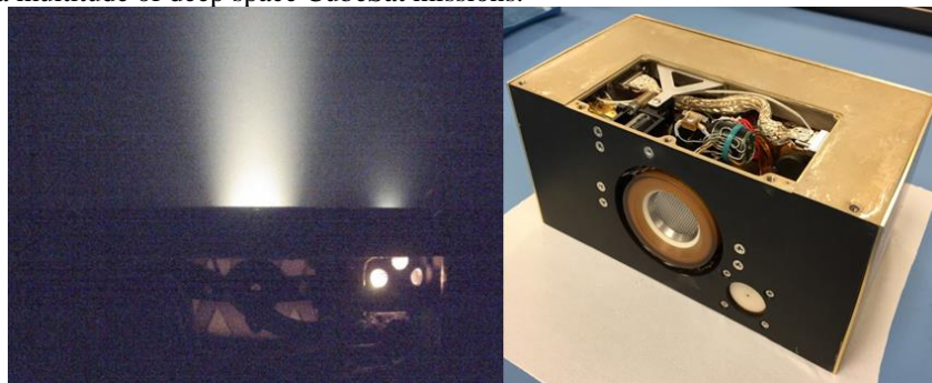
Figure 6: Integrated BIT-3 operating on iodine propellant (left); integrated thruster system (right)
