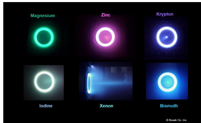
Figure 15: Alternate EP Propellants
