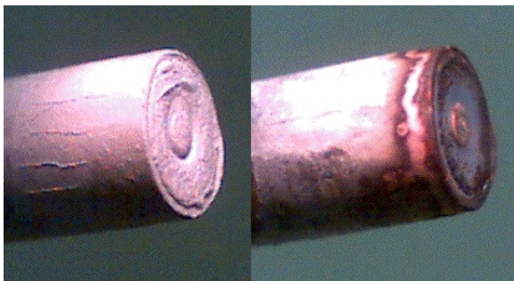
Figure 16: MicroPPT coated with barium hydroxide pre-firing (left) and after ~600 shots (right).
