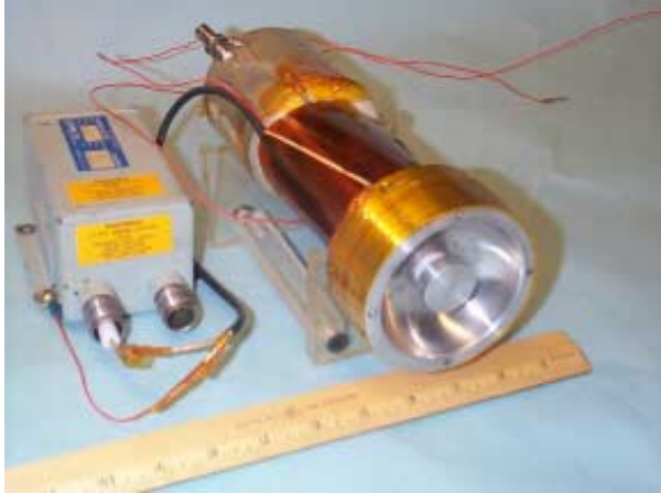
Figure 1: Picture of coaxial inverse-pinch PPT with the ignition circuit
