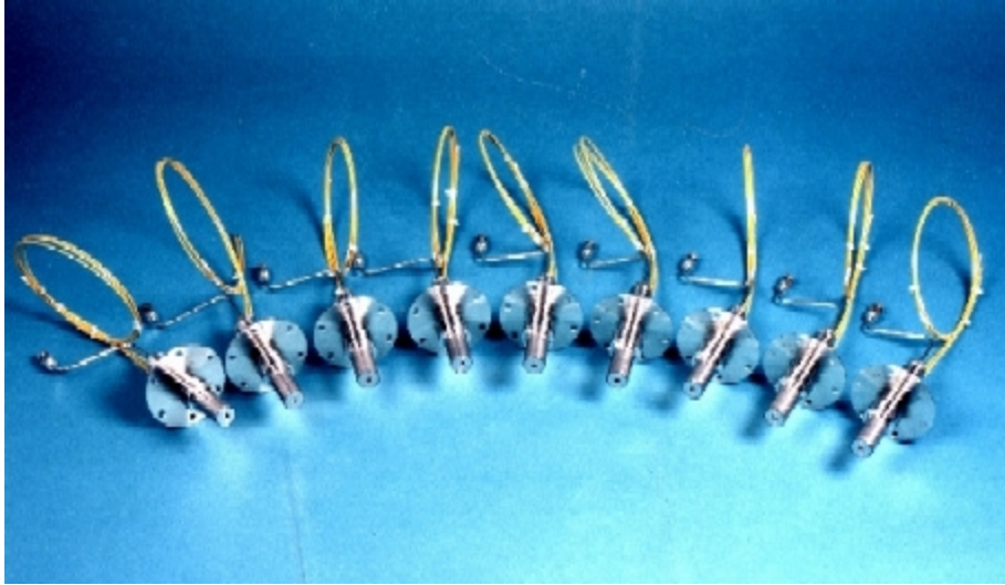
Figure 11. Photograph of 9 out of 12 flight HCA's designed and manufactured by NASA Glenn Research Center in support of the International Space Station plasma contactor program.
