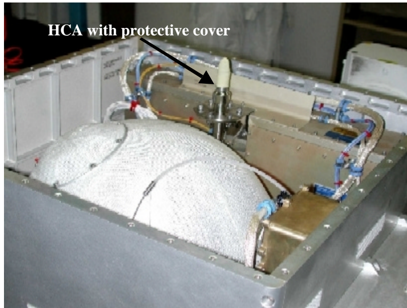
Figure 13. Photograph of flight HCA.004-F being integrated into the ISS PCU box. Image shows the PCU with its top cover removed. The large white sphere is the xenon storage tank. The HCA is pointed out in the picture.
