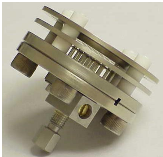
Figure 1 Photograph of the colloid source. The electrospray needles, and the extractor and accelerator electrodes can be seen in this view.
