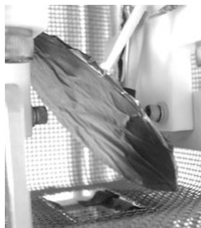
Figure 6. Close-up photograph of the detector plate housed within a Faraday cage.
