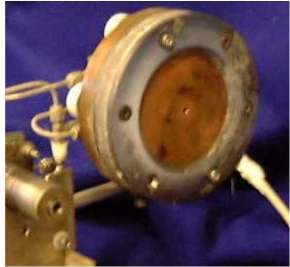
Figure 3. Photograph of the experimental setup for the arcjet neutralization studies. The arcjet shown in this photo is the higher power, nominally 1-kW laboratory thruster developed by NASA.
