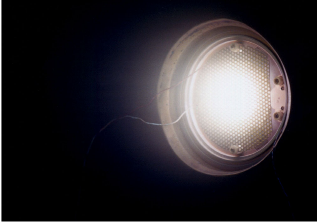
Fig. 3.3 Plasma snapshot (produced by microwave cavity with extracting grid)
