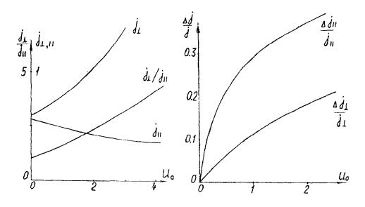
Fig. 2. Probe ion currents versus  $u_0$ ( $\phi_0$  =-6,  $\epsilon$ =1,  $r_0$ =3).
