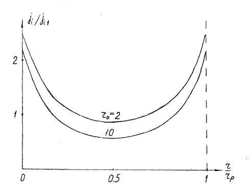
Fig. 1. "Edge" effect on ion current distribution.  $(\phi_0 = -20, \epsilon = 1, \ u_0 = 0)$
