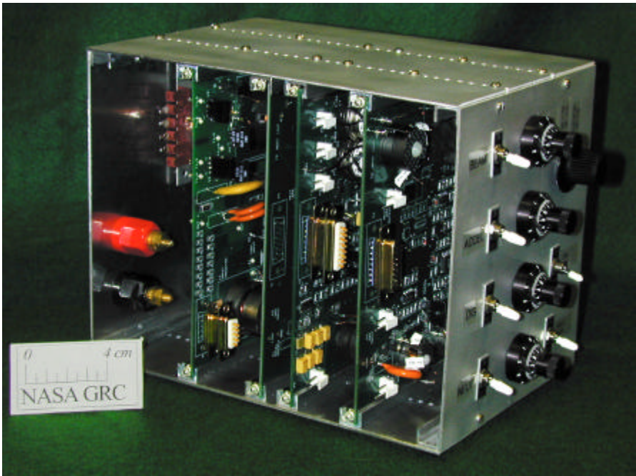
Figure 5 – Second-generation sub-kilowatt breadboard power processor unit.
