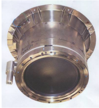
Figure 2. Photo of the ion thrusters RIT-22 manufactured by EADS Astrium ST. The standard engine's nominal operation performance data are: 175 mN thrust, 4760 s specific impulse, 5.83 kW power consumption, 3.72 mg/s propellant consumption.
