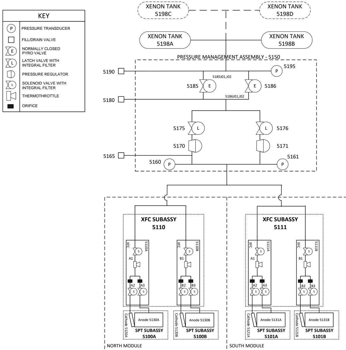
Figure 1. EP-140 subsystem pneumatic block diagram.
