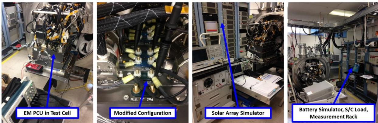
Figure 8. Psyche modified PCU test setup.
