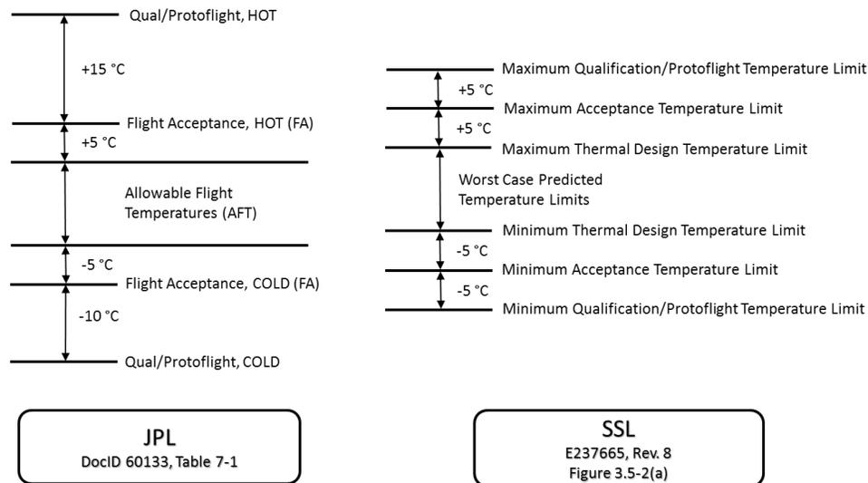
**Figure 2. JPL and SSL temperature margin comparisons for internally mounted and external thermally coupled equipment.<sup>6,7</sup>**
