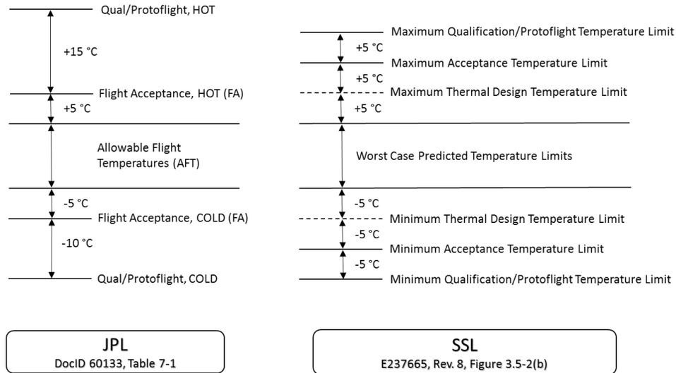
**Figure 3. JPL vs SSL temperature margins for externally mounted and thermally isolated equipment.**<sup>6,7</sup>
