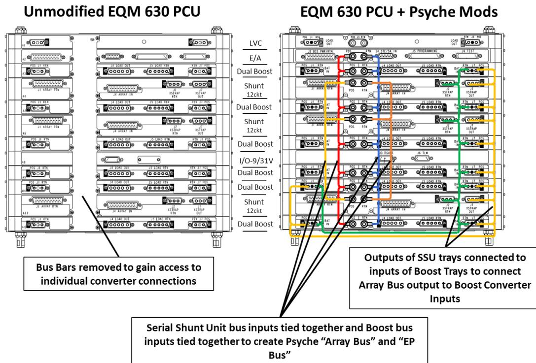
Figure 7. SSL comparison of heritage PCU and modified PCU outlining configuration changes for Psyche.
