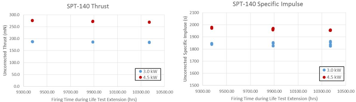
**Figure 5. SPT-140 Reference performance data during the life test extension operating at 3.0 kW and 4.5 kW.**
