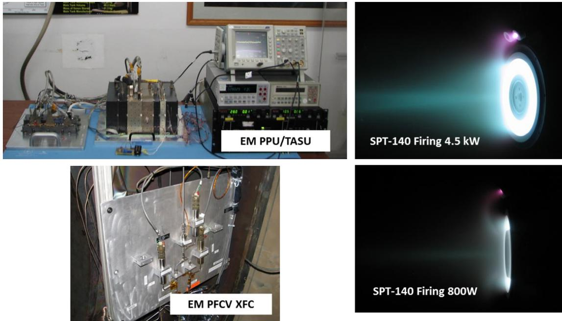
**Figure 6. SPT-140 operating at 800 W and 4.5 kW with engineering model (EM) PFCV XFC controlled by engineering model (EM) TASU & PPU.**
