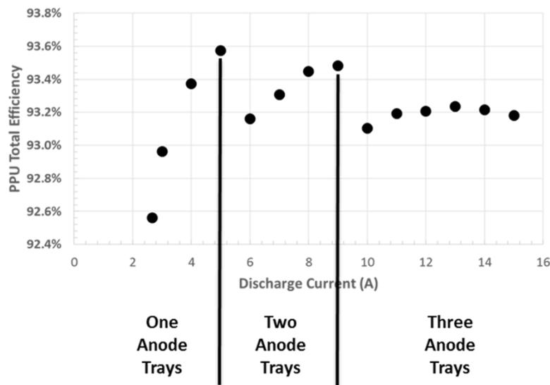
Figure 4. SSL PPU total efficiency as a function of discharge current.
